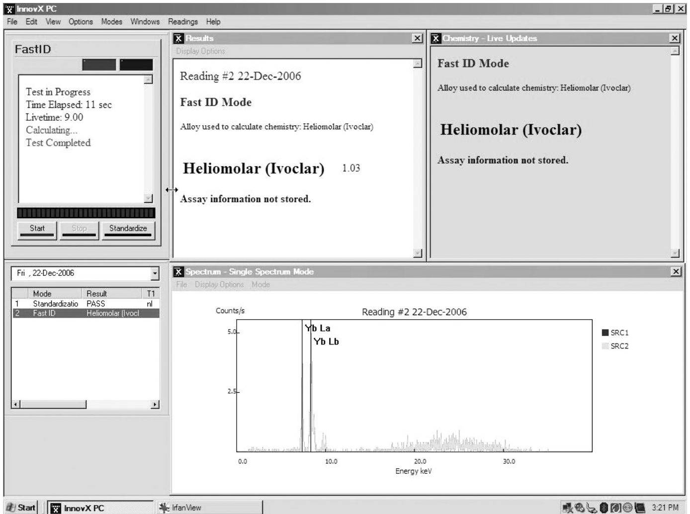
FIG. 3—Screen capture from analysis with portable XRF. The unknown is correctly identified as Heliomolar.
